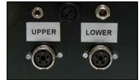
Rear-panel showing photo-detectors connectors.
